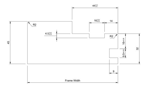
Do Not Scale. Description: Purchasing Profile Timber System 2 - 44\_32 Profile - FD30 - 45mm Door - Acoustic - Q2Flat To Pull
